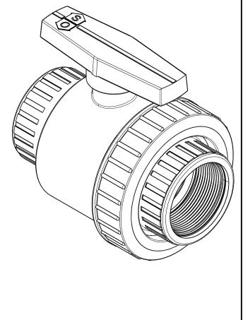
MATERIAL - POLYPROPYLENE WITH TEFLON SEATS EPDM O-RINGS
